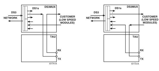
Figure 575-3e. Drop: Network / Insert: Customer
